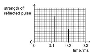
The speed of ultrasound in the metal is  $5000 \,\mathrm{m\,s^{-1}}$ .
